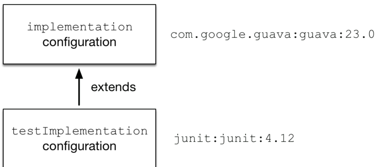
Figure 24. Configuration inheritance provided by the Java plugin
