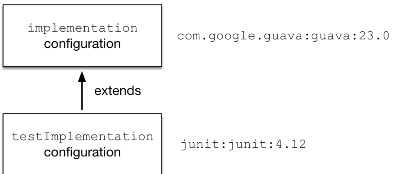
Figure 24. Configuration inheritance provided by the Java plugin
